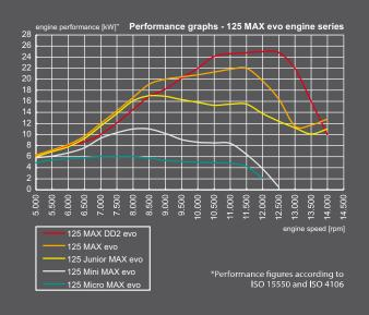
**Age** 8 – 10 years Race class mainly national **Maximum Performance** 6 kW / 8 hp at 7,500 rpm Maximum Torque 9 Nm at 6,000 rpm
